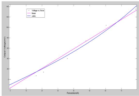
Fig. 10. linear and nonlinear fit on experimental data  $F_{mean}$  vs.  $V_{output}$
