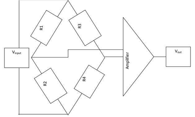
Fig. 2. Sensing Bridge Circuit
