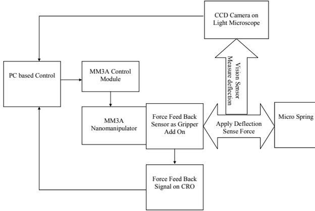
Fig. 3. Block Diagram of Complete Setup
