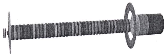
Figure 3. DC model of TWT
