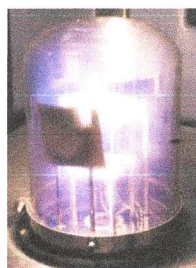
Fig. 1. : DC Triode sputtering set-up for triple alloy coating of CPD Cathode.
