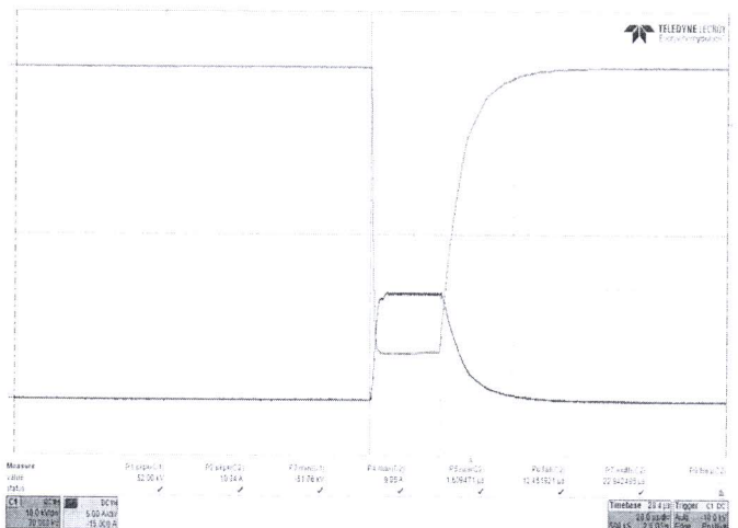
Fig. 15. -52kV, 10A pulse output waveform @20 \mu s, 200Hz Scale: X axis 1 unit=20 \mu s; Y axis 1 unit=10kV and 5A
