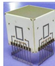
Fig.7: Alumina based module
