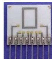
Fig.6: Alumina based package
