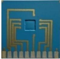
Fig. 3: Fabricated LTCC packages with inbuilt cavity
