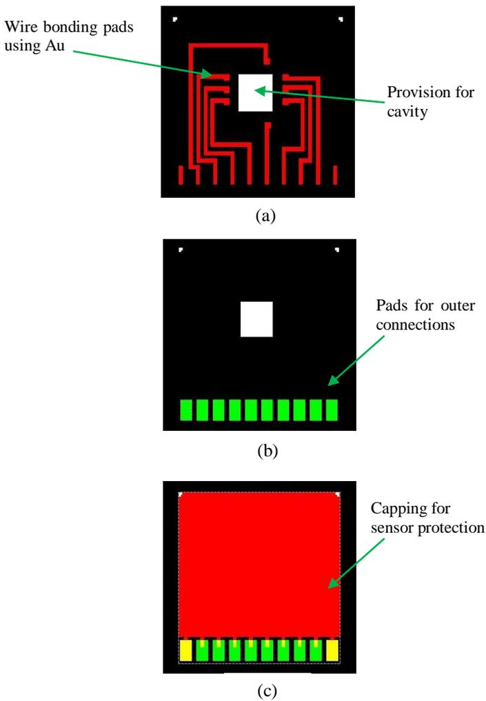
Fig. 1: Layout for eight pin configuration
