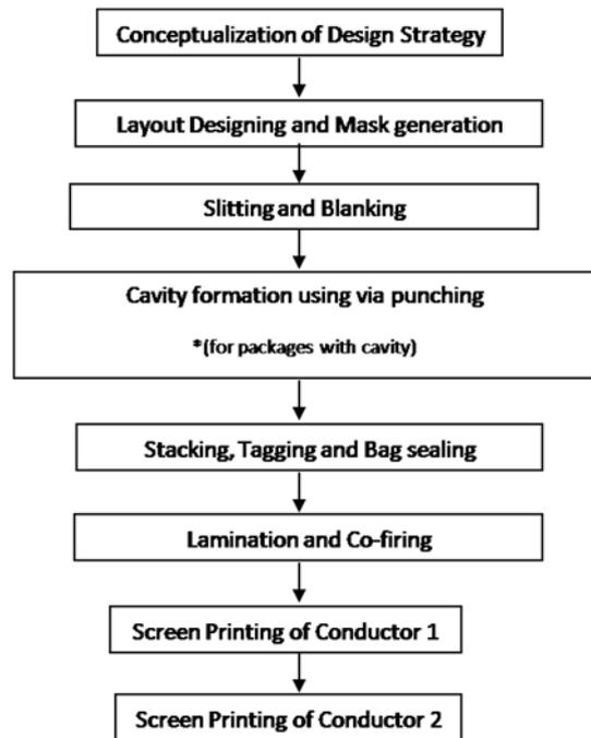
Fig. 2: Fabrication Process Flowchart
