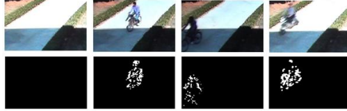
Fig. 4. Moving Objects in Video Scene and Corresponding Motion Detected Outputs for Pseudo-stationary Background Scenarios.
