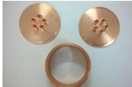
Figure 4. The piece parts of a five beam cavity
