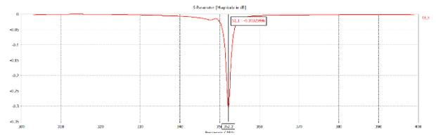
Fig.7 Plot of S11 parameter vs Frequency
