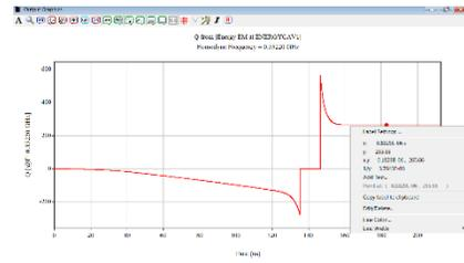
Fig.5 Simulation of the External Q parameter
