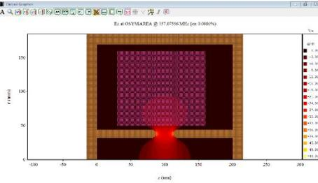
Fig.8 Simulation of third cavity at 357 MHz
