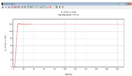
Fig.10 Simulation of 'R over Q' at cavity gap
