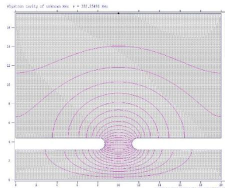
Fig.2 Simulation of input cavity in SUPERFISH
