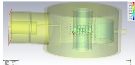
Fig.6 Simulation of the input cavity with coupler
