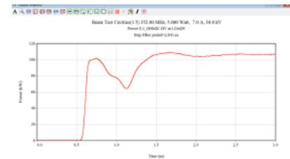
Fig.14 Simulated output Power in MAGIC
