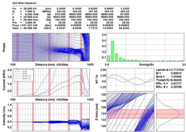
Fig.3 Simulation through AJDISK code
