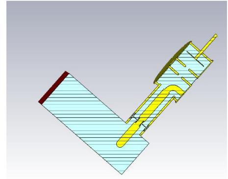
Fig. 11 Simulation of the output cavity
