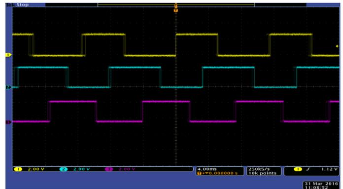
Fig.23: Hall waveform from Hurst BLDC motor
