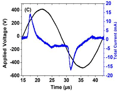
Figure 2.(a)Filamentary and Homogeneous discharge,(b) I-V Characteristic
