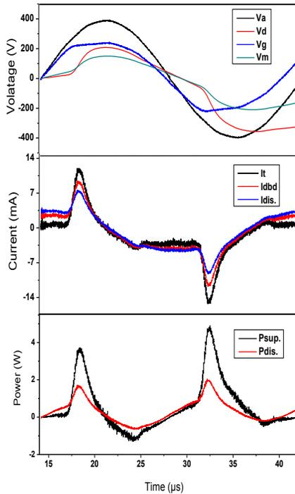
Figure 3 Experimental waveforms of dynamic processes occurring in gap (gas: Helium at  $f = 34.5$  kHz) for the Parallel plate DBD Geometry. at 100 mbar.
