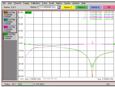
Figure 5. Measured Return Loss & Insertion Loss of the window.
