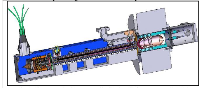
**Fig.8: Systematic diagram of a high efficiency space TWT**
