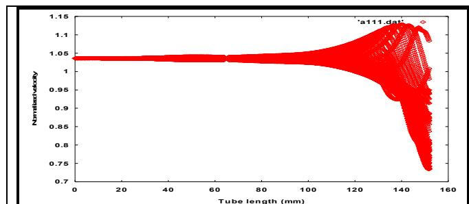
**Fig.6: electrons velocities using SUNRAY-1D for a space TWT operating at saturated drive power**
