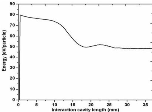
Fig. 3: Profile of electron energy in the interaction cavity for  $TE_{28,7}$  mode gyrotron
