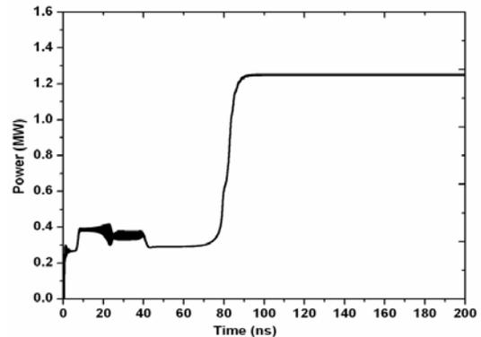
Fig.1: Output power for TE<sub>28,7</sub> operating mode gyrotron at the fundamental harmonic number
