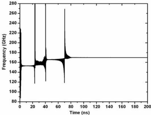
Figure 2: Frequency as a function of time for  $TE_{28,7}$  mode gyrotron
