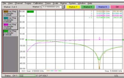
Fig 4 Measured Return Loss & Insertion Loss of the window.
