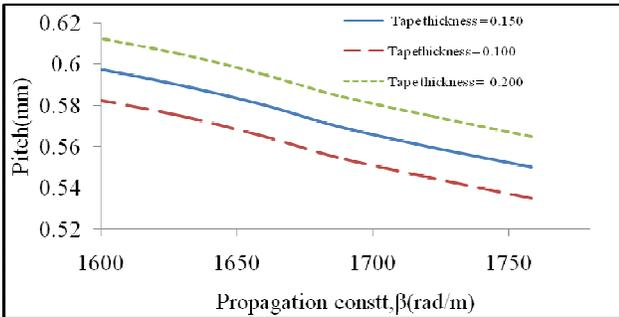
**Figure 3.** Pitch(mm) vs.  $\beta$  at different Tape thickness
