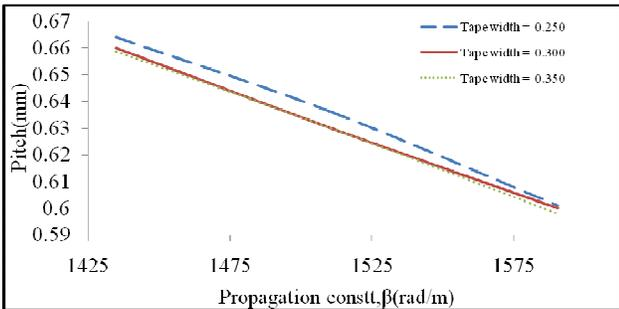
**Figure 5.** Pitch(mm) vs.  $\beta$  at different Tape width
