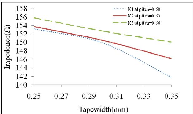
**Figure 7.**  $K(\Omega)$  vs. Tape width(mm) at different  $\beta$
