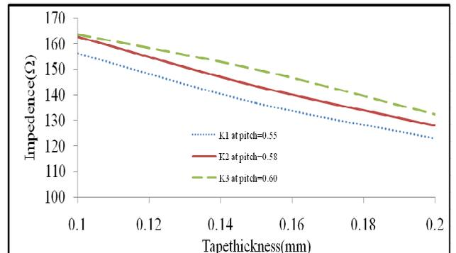
**Figure 8.**  $K(\Omega)$  vs. Tape thickness(mm) at different  $\beta$
