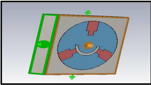
**Figure 1.** CST-MWS model of helix SWS
