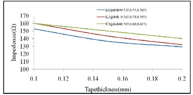
**Figure 4.**  $K(\Omega)$  vs. Tape thickness(mm) at constant  $\beta$
