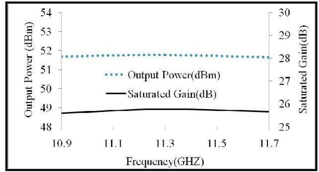
**Figure 2.** Power(dBrn),Gain(dB) vs. Frequency(GHz)
